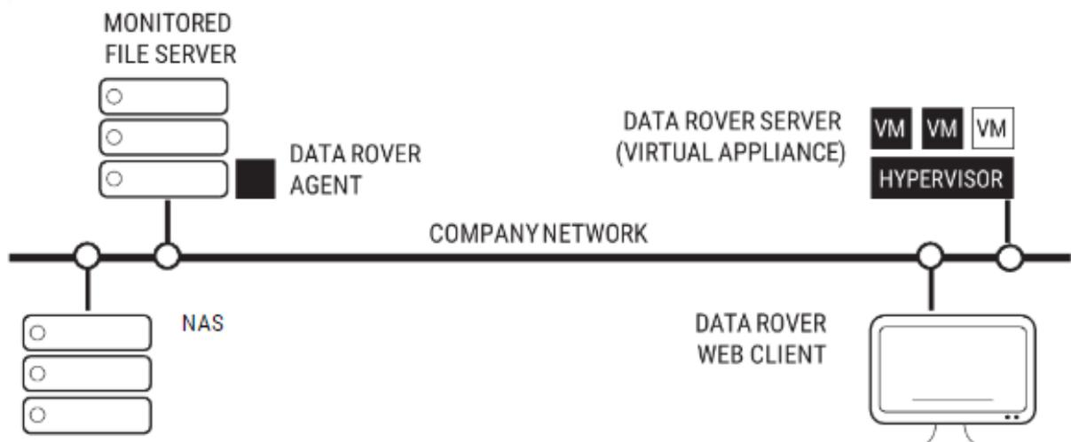
In the diagram above, we see a typical Data Rover installation. The Data Rover server is located within the customer's virtual infrastructure. Monitoring of storage resources (File Server or NAS) takes place via Agents. The Agent can be installed natively on Windows-based file servers or on a support service machine to scan NAS devices.
