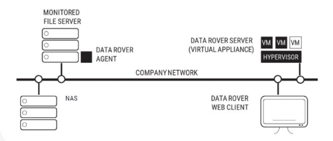
In the diagram above, we see a typical Data Rover installation. The Data Rover server is located within the customer's virtual infrastructure. Monitoring of storage resources (File Server or NAS) takes place via Agents. The Agent can be installed natively on Windows-based file servers or on a support service machine to scan NAS devices.
